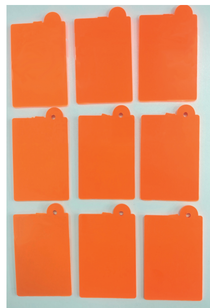
Fig. 3. Sample body in orange color after temperature storage test. © Ascend
